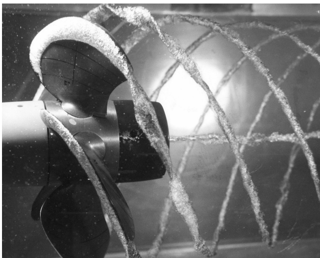
Figure 1.5: Leading edge-tip vortex cavitation, from [26]
