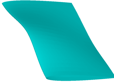
Figure 5.2: Surface geometry of Twist 11 hydrofoil. \alpha_{max} = 11 degrees and \alpha_{wall} = -2 degrees
